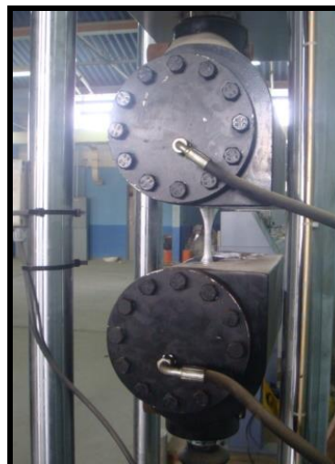
Plate (3) Test setup of aluminum tensile coupons
