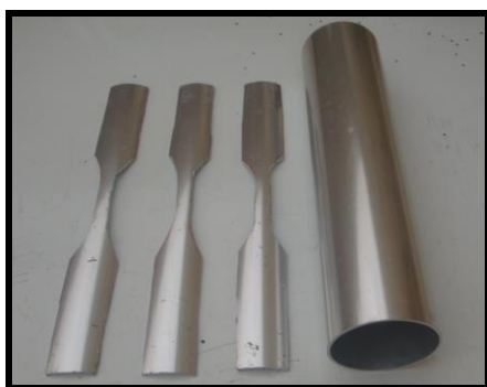
Plate (2) Aluminum tensile coupons
